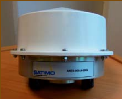
GARDA antenna pre-industrial prototype covered by its radome
