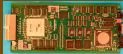
GARDA Receiver DSP Board
