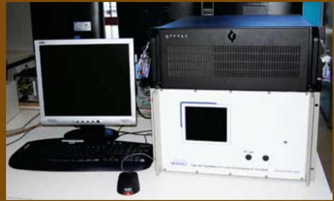
(above) Prototype Galileo Simulator used for Rx functional & performance tests (left) Vector Signal Generator used for Rx boards tests
